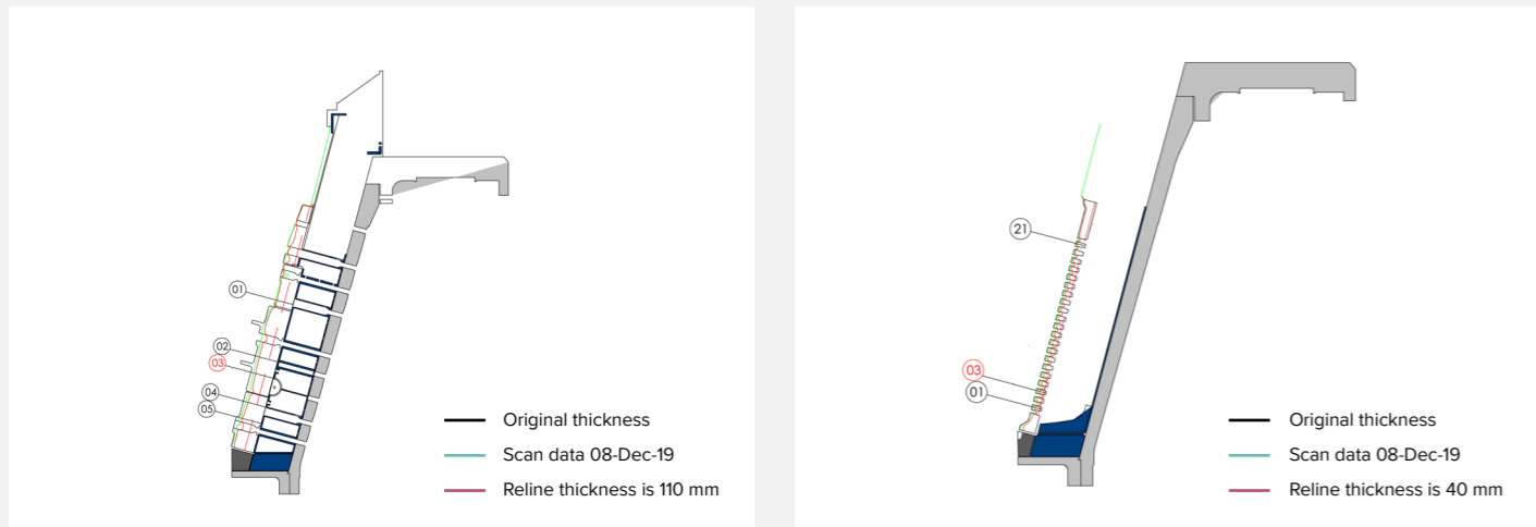
Discharge head grate longitudinal lifter & plate as on December 08, 2019
