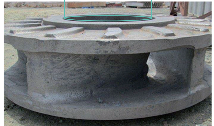
millMAX pump impeller eye is protected from recirculation wear by the wear ring
