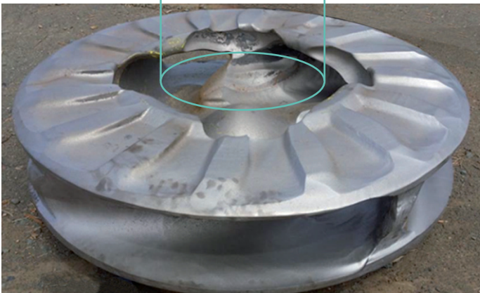
Competitor's pump impeller eye is enlarged and deformed, indicating suction-side recirculation
